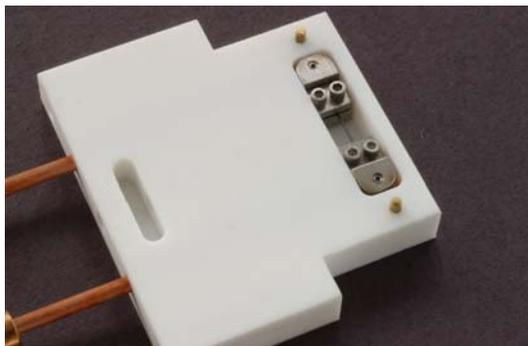
Fig. 4 Original Ion Source (less metallic shield)
