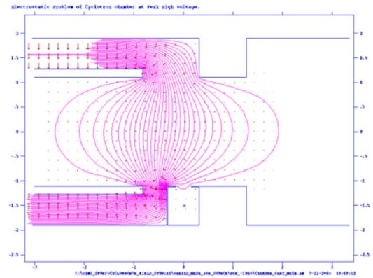
Fig. 5 PSF model showing suppression of e-
