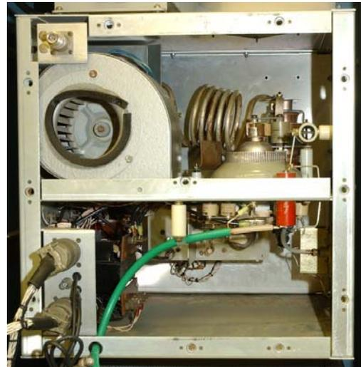
Fig 16 Opened view of RF amplifier
