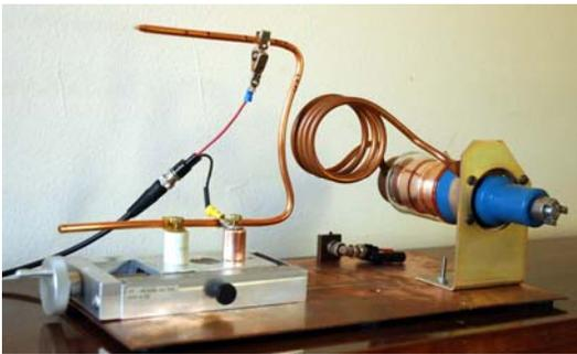
Fig.11 Cyclotron RF simulator
