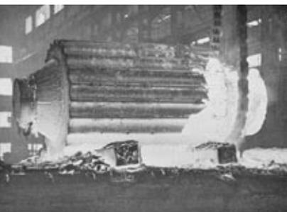
The magnet originally was part of a particle accelerator known as a synchrocyclotron. Electric fields propelled particles and the magnet bent their path. The particles cycled between the two poles of the magnet until their speed was great enough for producing high-energy collisions. The first accelerator of this type began operating in November 1946, at the University of California, Berkeley.
